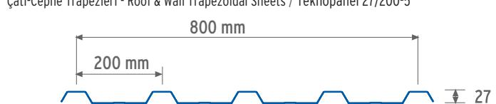
Çatı-Cephe Trapezleri - Roof & Wall Trapezoidal Sheets / Teknopanel 27/200-6
